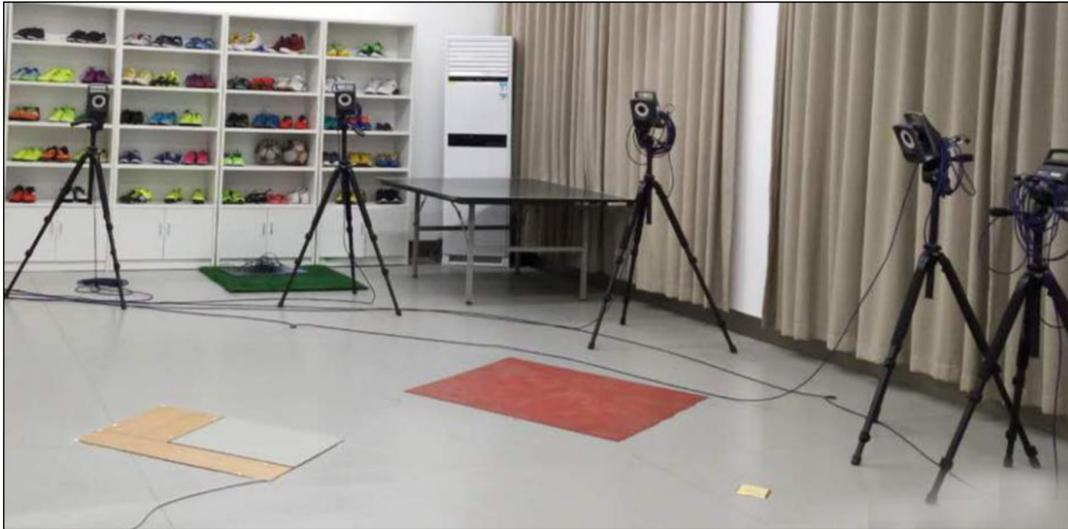
**Figure 3:** The 8-camera Vicon motion analysis system (Oxford Metrics Ltd., Oxford, UK).
